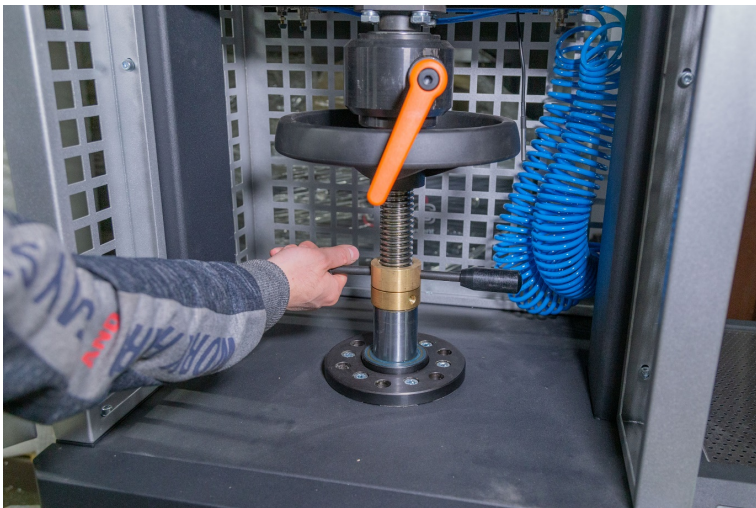
Figure 23. Loosening the lower clamp height adjustment stopper
