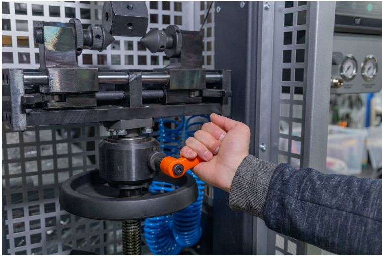
Figure 22. Loosening the bottom clamp stopper
