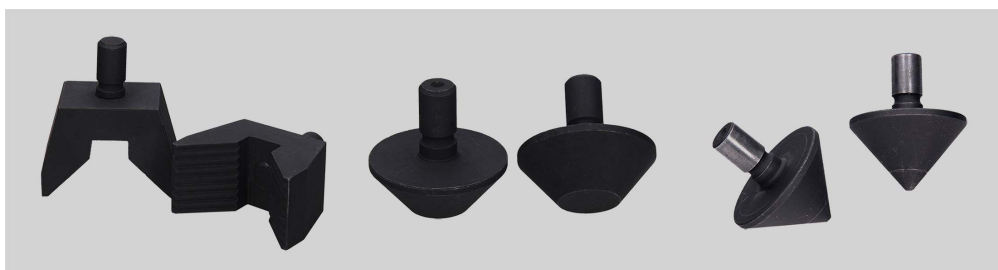
Figure 2. Shock absorber changeable fittings for lower pneumatic clamp (for various types of shock absorber mounting mechanisms)
